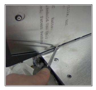
10)Next, connect both R legs (with wheels). If already attached, the wheels should face outward. Start each of the three long Philip's self-tapping screws – make sure they are through the leg and properly aligned, then use a variable-speed drill with a Philip's bit to start them. Finish tightening with a
