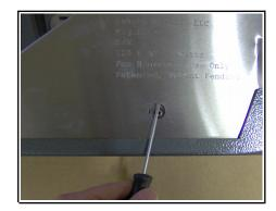
5) Align the R (right) shelf and place two hex-head ¼" bolts in the right (back) slots; finger tighten. Insert the other two bolts and finger tighten. Once all four bolts are started, use a 7/16" wrench to tighten them.
