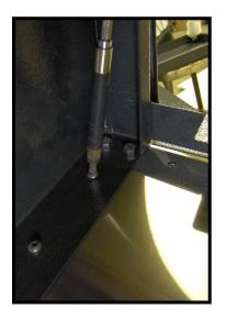
6) Insert 2 Philip's self-tapping screws into the R shelf. The R shelf is now in place.
