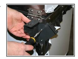
3. Open the *Lid* and attach the *Lid Handle*, as shown at right, using four self-tapping screws.
