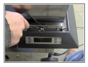
8. Attach #6 nuts on back. (Same as Step 4). Finger tighten.
