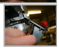
Finger tighten as much as possible, then snug the nuts a bit more with a pair of needle-nose pliers. *Caution: do not over tighten!*
