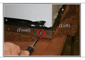
4. Second, attach the middles of the two *Back Legs*, as shown below, with three self-tapping screws apiece. Do not put screws in the bottom two holes at this point. Again, you may need to "lever" each leg as you attach the screws. *Note: Once the first screw is in, you may tighten it to hold the leg in place.* The *Back-Left Leg* is shown.
