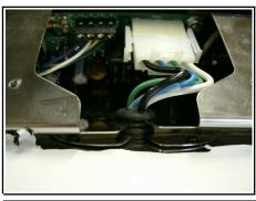
16. Attach S/N Cover using 2 #6 Self-Tapping Screws.
