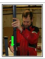
Note: the tab on each leg will be against the front or back of the grill (not against the sides).
