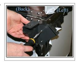
9. Open the *Lid* and attach the *Lid Handle*, as shown at right, using four self-tapping screws.
