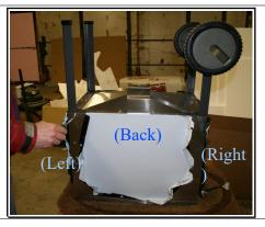
5. Third, attach the *triangle pieces* of all four legs, as shown at right, each with two self-tapping screws.
